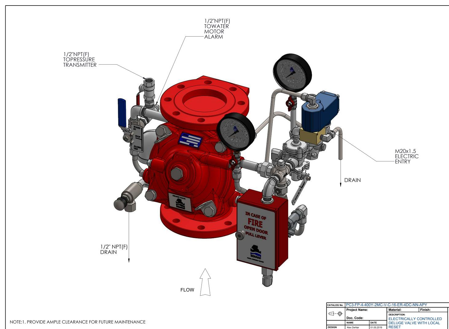
SCALE: 1:3 A3 SHEET 1 OF 2 REV. 0
