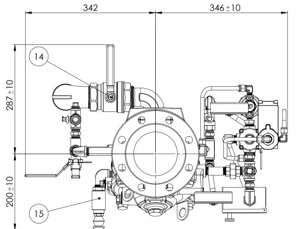
PC3-FP-4-400Y-2MC-V-C-16-ER-4DC-NN-APY CATALOG No. Material: Finish: Project Name: €--DESCRIPTION: Doc. Code: ELECTRICALLY CONTROLLED DELUGE VALVE WITH LOCAL NAME DATE **RESET** Alex Dehtar 01.05.2019 SCALE: 1:5 A3 SHEET 2 OF 2 REV. 0 File name: PC3-FP-4-4 DRAWN Alexander Bezrebriy 01.05.2019 APPROVED Alex Dehtar DWG No.022278 WEIGHT [Kg]:55 07.05.2019
